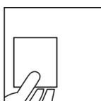
Test spray after shaking the can - Compatibility with the respective substrate as well as Check hue.
