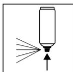
After finishing the painting process can turn over and spray valve empty to turn on to avoid sticking of the spray valve.
