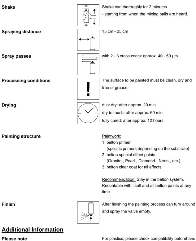
heck and prime with belton basic plastic primer. Do not spray on synthetic resin painted surfaces, as the paint may pull up.
